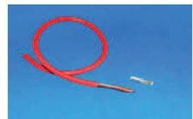
PP contact and crimp or solder in place. I like using the West Mountain Radio ratcheted crimper as it is positive, and quick. Cut the wire about 1 1/2 inches long and repeat until you have seven Red and Black wires with PP contacts attached.
