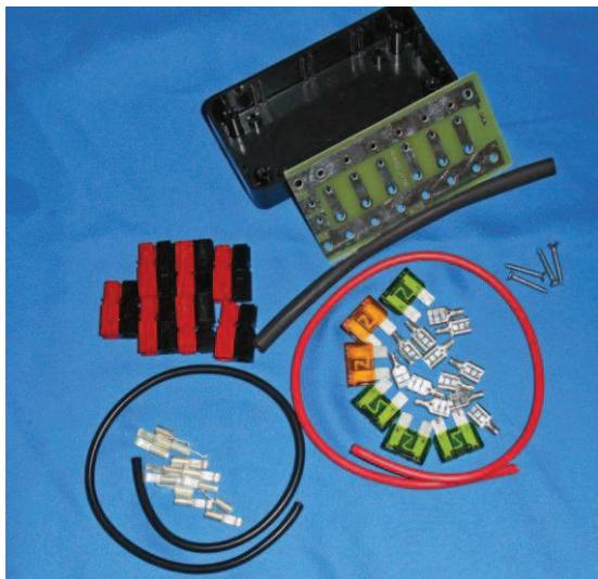
Gather all the parts for the project sort them in separate containers. I find that the aluminum "Throw-away" muffin tins are ideal for small projects and inexpensive. Examine the PCB for errors, flaws and make sure the holes are all drilled and correctly sized for the components.
