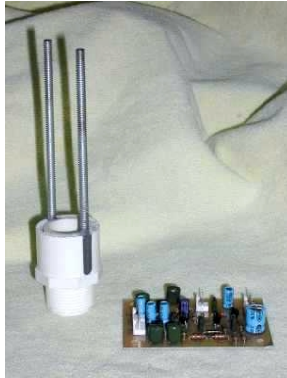
3/4" Adapter with All-Thread Epoxied in Place
