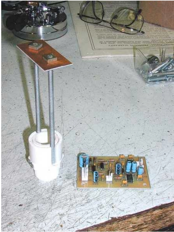
3/4" PVC Adapter with All-Thread Set in Place Note the support plate for the All-Thread
